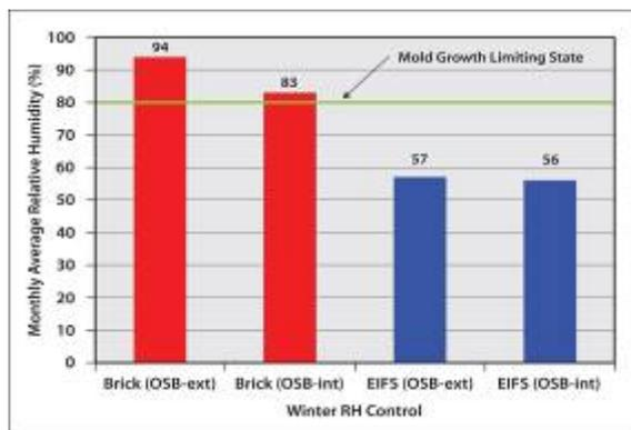
*Controlling humidity at the oriented strand board (OSB) sheathing is key to controlling mold.*
