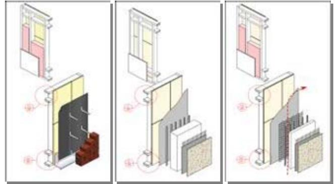
*A conventional wall composed of brick façade on wood frame was tested alongside various EIFS walls. The drawings in the middle and on the right above are EIFS designs that have proven superior in both moisture control and insulating value.*
