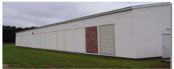
The EIFS Industry Members Association underwrote the cost of a natural exposure test facility in Charleston that can test 15 different wall systems side by side.
